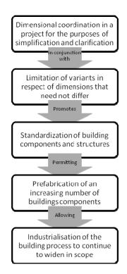
Figure 1: Concept of non-traditional construction methods. Adopted from Nissen (1972)
